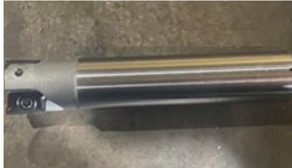
Gambar 5. Hasil rancang bangun holder square shoulder
