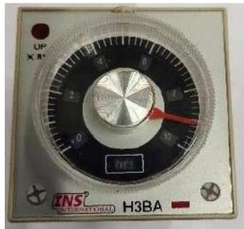
Gambar 2. Time delay relay
