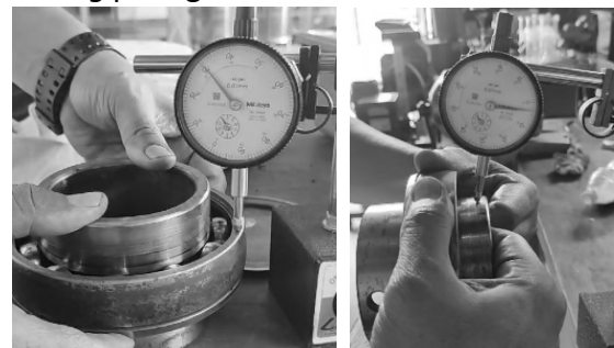
(a) (b) Gambar 3 . Pengukuran Clearance Bearing a) Aksial b) Radial
