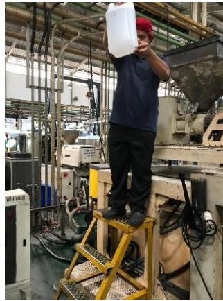
Gambar 4. Uji drop test
