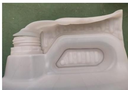
**Gambar 5.** *Poor handle trimming*
