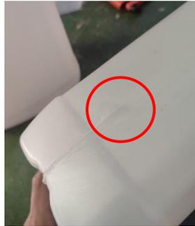
**Gambar 9.** *Flashing*
