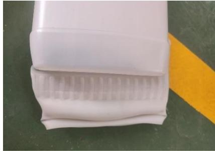
**Gambar 6.** *Poor bottom trimming*
