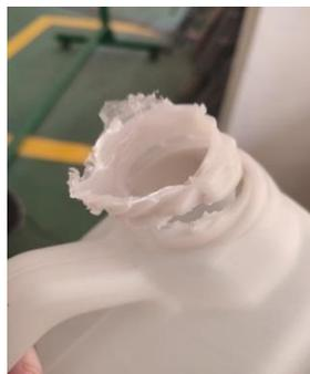
**Gambar 7.** *Poor trimming*
